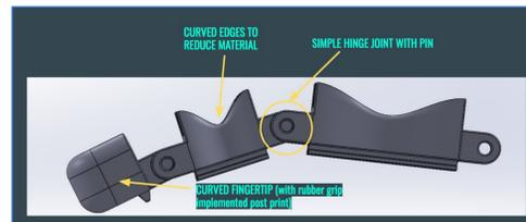
**Figure 3.1: First Prototype Model**
