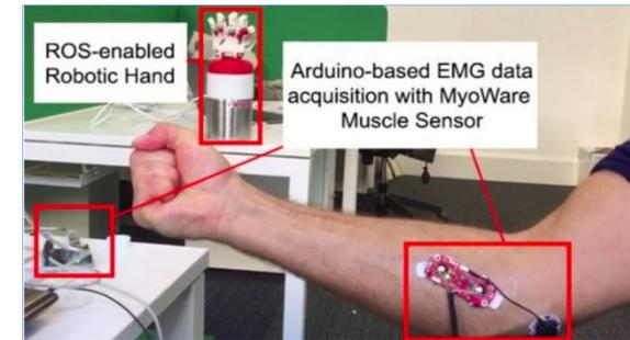
**Figure 8: Electromyogram Control**
